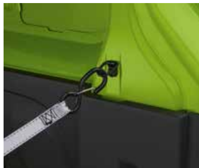
16 anchorage rings as standard on SWB, 18 on LWB versions
