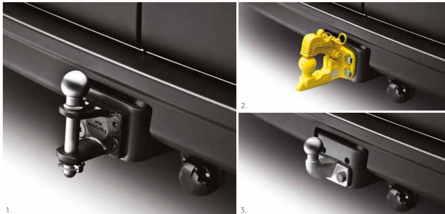
TOWBARS 1. Universal Coupling 2. 'Pintle Hook' with ball 3. Standard Ball: Renault goes above and beyond even the strictest European standards (CE 94/20). Thanks to further testing, Renault have also made sure that your vehicle won't be damaged, even with intensive commercial towbar use. Renault also take the most demanding climatic conditions into account by applying an anti-corrosion surface treatment. A range of different tow balls and hitches are also available
